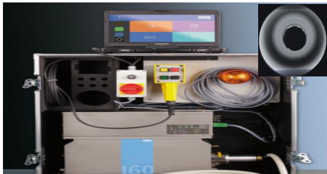
RT on Tube-to-tubesheet Joint
