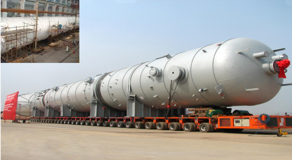
PDH Project- Thailand – CTCl; DN5100*70000, CS, 580ton
