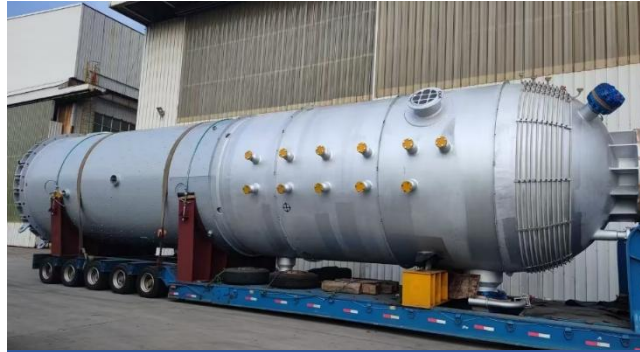
Cyclohexanone Plant - Reactor DN3400*3/110*18000 139 ton (C276/CS Clad)
