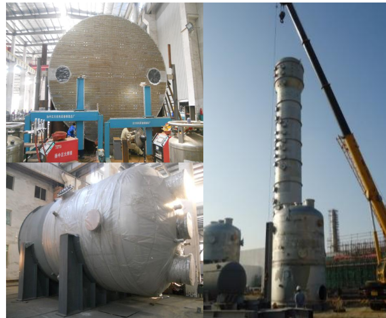
Formaldehyde Synthesis Reactor DN4924*8450mm, 58tons 17,400 tubes, SS304, Tubesheet 50mm
