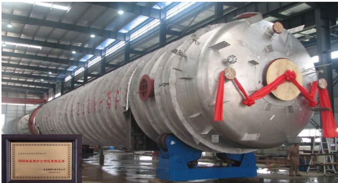
Acetate Project Prime Distillation Column DN3985 * (8~12), L=34000mm N08020
