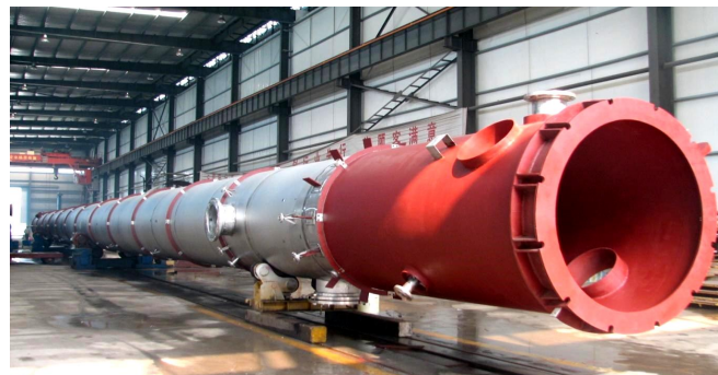
Column for Acetic Anhydride Project DN1600*41850; N10276
