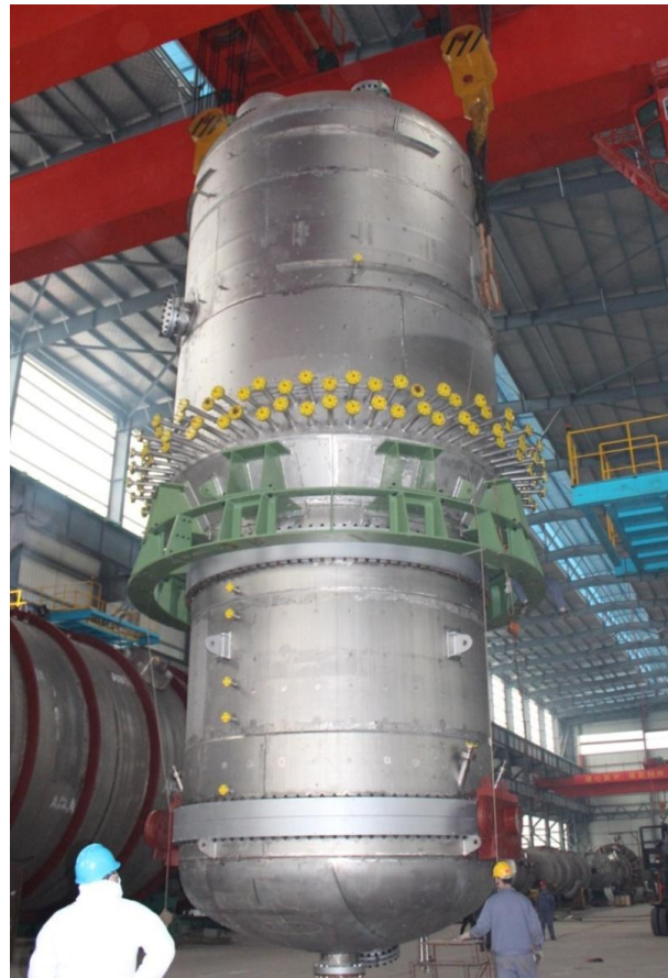
OC Reactor Thailand – MES - 2014 Indonesia – Uhde - 2015 Hungary – BorsodChem - 2025 DN5800; 250tons SS304, N10276, CS
