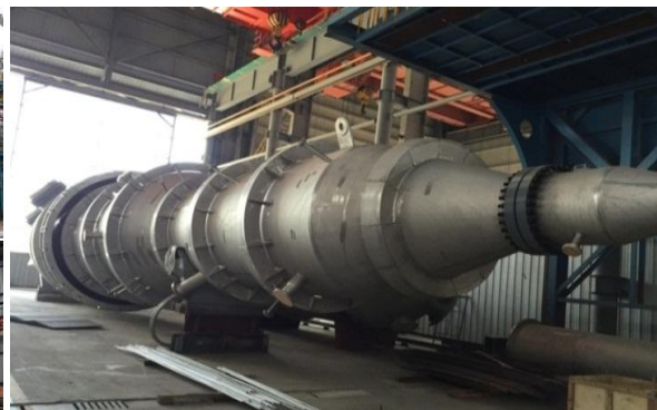
UOP PDH Project Regeneration - N06600 DN2740
