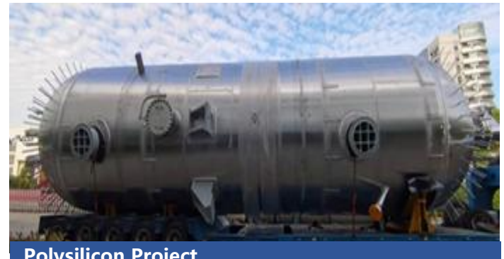
Polysilicon Project Fluidized Bed Reactors (800H, 8120) DN4500*90*23000, 255ton
