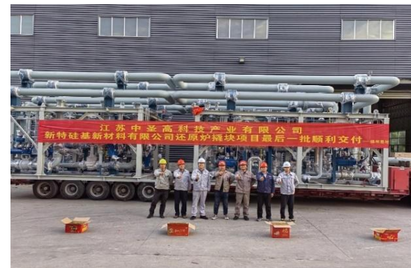
Polysilicon CVD Reactor Skid
