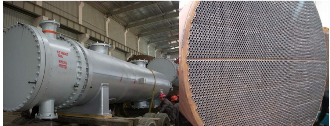
UOP Process PDH Project - High Flux Tube Heat Exchanger CS, Copper Alloy Material (Thailand, Canada)
