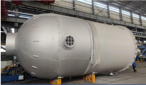
Cyclohexanone Plant – Reactor DN5000*3/170*12600 188 ton (C276/CS Clad)
