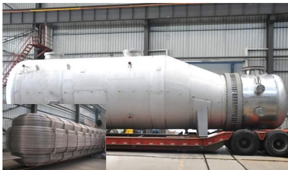
Energy Recovery Project DN3200; N10276
