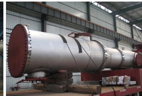
Fluorine Chemical Project DN2600*41850; N08825
