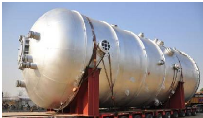
Oxidizing Reactor DN7300mm;Ti+CS
