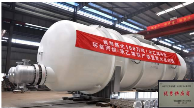
1,000,000t/year Ethylene Project – PO/SM Unit Dehydration Reactor DN4300*15000, 103tons, N08020
