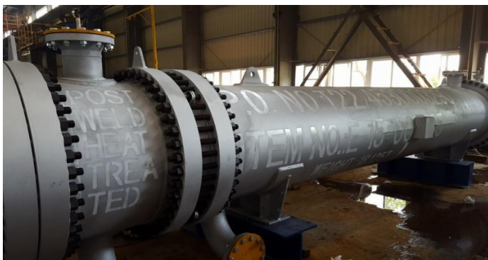
AS Helix Heat Exchanger / SA516 Gr.70
