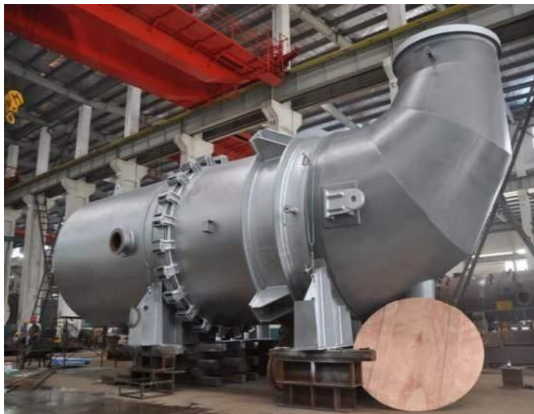
1st, 2nd & 3rd Effect Evaporation Reboilers Glycol EO/EG Project DN4000, 150tons, SB111 C70600 B10
