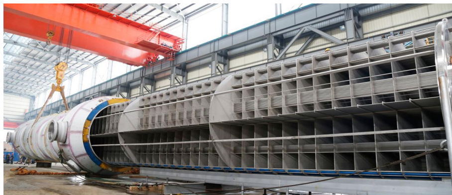
MEGlobal BOOKRAMEG Project USA, 19 Items (Column+HE); DN5200, L=29m, 800ton, SS304L
