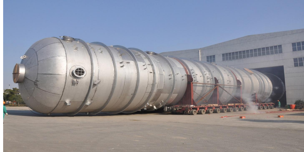
HengLi Petro Chemical; Dehydration Column; DN8800*47200; 328.5tons; Duplex S32205
